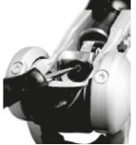
Fig 4. Remove head cap screw
