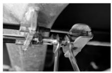
Unscrew push rod from brake rod and slide it from the guide tube. Remove the locking nut from push rod using two 17mm spanners.
