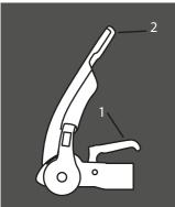
Figure 7 - Raise stabiliser lever
