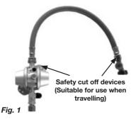
Approved for en-route heating if your caravan has a factory fitted habitation en-route LPG heating system that can be used whilst travelling. Fig 1 shows the two safety valves features that are part of the system, these are there for your safety whilst using the system when travelling. When in use ensure all other gas appliances are separately isolated.
