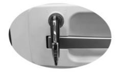
There are 3 primary positions for the internal handle inside the caravan, these are locked, neutral and open. When closing the door from the inside the caravan ensure the handle is in the neutral position, The handle MUST NOT be partially up in the locked position as this will prevent the door from closing causing damage to the door
