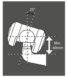
*Figure 2* - Max suitable rotation of overrun device is 25°.
