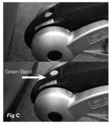
The hitch head is fitted with a visual indicator to show whether or not it is properly connected to the towball. A green band will show immediately below the red indicator button on the hitch head when a proper connection has been made. (See Fig. C)
