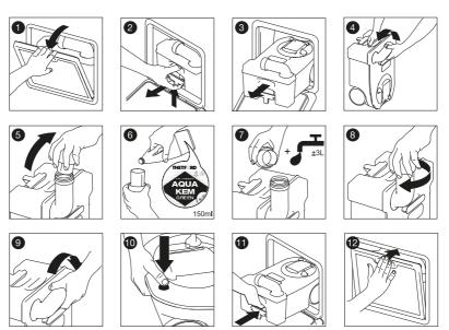
Preparing flush-water tank (only for C262-models)
