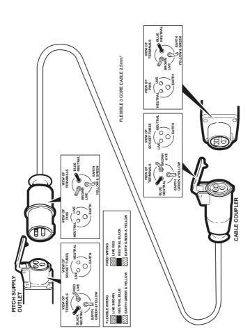
WIRING OF CONNECTING CABLES AND CARAVAN MAINS INLET
