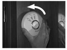
Remove the existing battery and replace with a new battery. From the list above, making sure that the positive and negative connections are in the correct position. If unsure see the alarm user manual.
