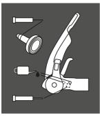
A WARNING: When lubricating, ensure none gets into the friction pad or towball holding area.
