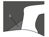
Fig 2. wear indicator - good condition
