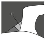
Fig 1. Wear indicator - good condition
