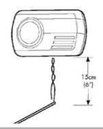
**Note:** We suggest the use of an incense stick or cigarette as the way in which these products burn produces a readable localized amount of CO. A readable level of carbon monoxide will not be given off by other sources of smoke, for example an extinguished candle or match.
