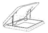
Forced ventilation functions via a brush lined duct instead of a ventilated pane.
