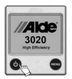
The system will now be drawing variable 0.2–1 A of current from the 12v supply.
