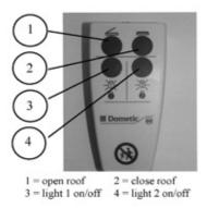
By short pressing the button 1, the glass dome will be opened up to 70 degrees. Should an opening up to 70 degrees not be required, this could be interrupted by pressing the button 1 once again. Press the button 2 permanently for closing the roof until the desired position is reached. The control lamp is switching off when the glazing panel is completely locked.
