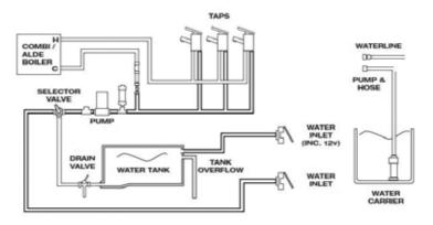
• Two water inlets are fitted on the outside of the caravan, on the offside. The upper inlet is used to fill the internal water tank, and the lower inlet is used to bypass the tank.
