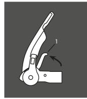
Figure 8 - Pull coupling handle up
