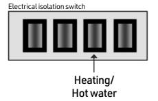
The Orange 230V / Mains isolation switch on power supply unit must be ON / illuminated for electric operation of the Alde central heating system.
