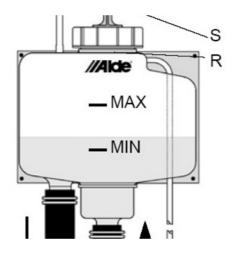
The Alde 3020HE central heating system can provide hot water and room heating, from gas and/ or mains (230v) electric energy sources. The room heating can be used with or without water in the heater - if water is present, then the water will also be heated to an unspecified temperature..
