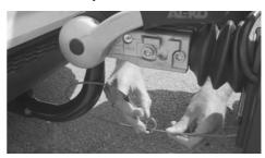
Align the 13 pin plug with the receiving socket on the tow vehicle.
