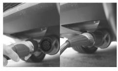
Insert & twist road lighting connector (13 pin plug)
