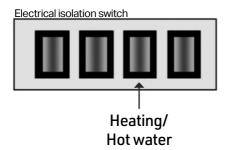
The Orange 230V / Mains isolation switch on power supply unit must be ON / illuminated for electric operation of the Combi.
