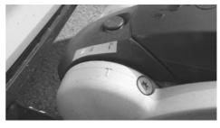
Ensure breakaway cable is attached.
