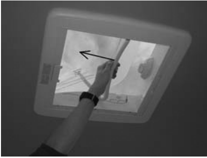
Pull the bar down and forwards ( Fig. B ).
