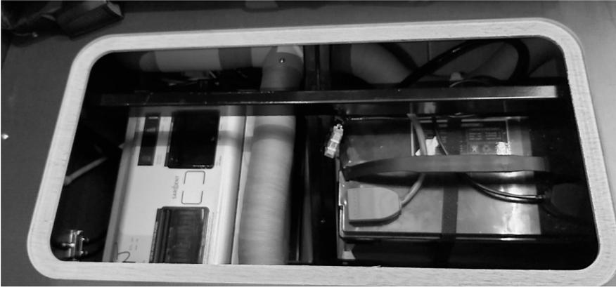
The battery is held in place by a tie-down strap that loops over the top of the battery.
