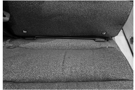
Top tether anchor points are fitted on the upper seatbelt stanchion and are accessed by removing an insert on the backrest cushion.
