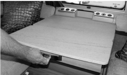
**⚠ WARNING:** When erecting the free standing table, be careful to avoid trapping fingers.
