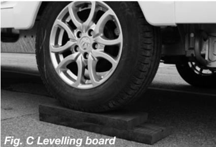
*Fig. C Levelling board*
