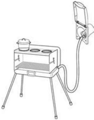
When external gas equipment is being connected, the operating pressure of the gas supply of 30 or 50 mbar must correspond with the operating pressure of the equipment that is being connected (see data plate).
