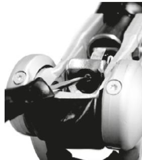
**Figure 19** Remove head cap screw
