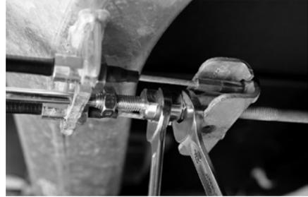
Unscrew push rod from brake rod and slide it from the guide tube. Remove the locking nut from push rod using two 17mm spanners.
