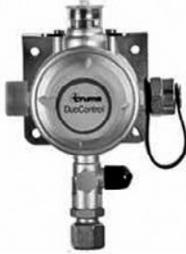
The DuoControl combines the gas pressure regulator and the changeover valve in one unit for operation as a two-cylinder system. When the operating cylinder is empty, DuoControl automatically changes over to the reserve cylinder.
