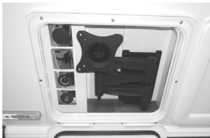
An external service door positioned on the door side of the caravan houses the connection points and an extended vesa bracket to mount a TV for viewing inside the awning. This comprises 230v & 12v sockets, aerial points and the TV bracket.
