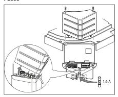
The water heater 12 V fuse is on the electronic control unit on the water heater.
