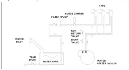
When power is supplied to the pump, it will draw water from the water tank, and pump it to the motorhome taps, shower and water heater.
