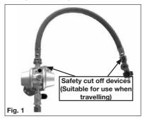
Your vehicle is supplied with a wall mounted gas regulator plumbed inside the gas bottle compartment. The regulator and all appliances work at a harmonised 30mb pressure, which work with Butane and Propane gas.
