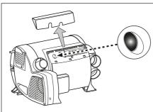
To reset the overheating protection, allow heater to cool, remove connection cover and press red reset button.
