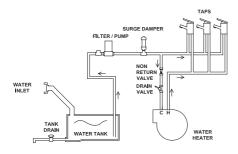
When power is supplied to the pump, it will draw water from the water tank, and pump it to the motorhome taps, shower and water heater.
