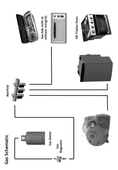
Typical gas schematic drawing with combi boiler
