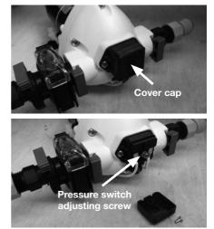
The pump may have to be removed to gain access to the adjusting screw. Drain the water system before removing the pump.
