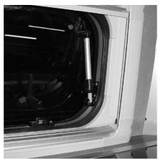
To open, turn knobs anti-clockwise and open catches. Swivel the window pane open to the desired position and close knobs clockwise to lock in the open position.
