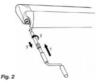
Unroll the awning while keeping the crank down. The awning will only open after a couple of turnings.
