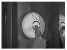
2. The unit will emit a loud (85dB at 3 meters) alarm for around 5 seconds and stop automatically.
