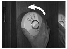
2. Remove the existing battery and replace with a new battery from the list on the previous page, making sure that the positive and negative connections are in the correct position. If unsure see the alarm user manual.
