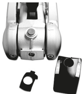
Figure 18 Cheese head screw revealed
