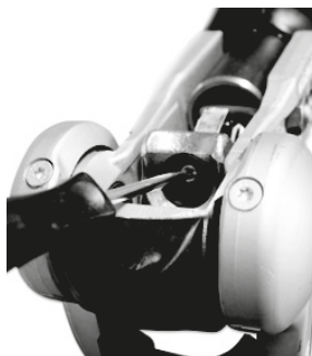
Fig 19 Remove head cap screw
