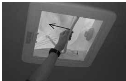
Pull the bar down and forwards (Fig. B).
