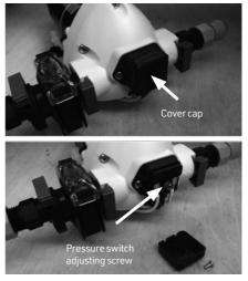
The pump may have to be removed to gain access to the adjusting screw. Drain the water system before removing the pump. To remove the pump pull the blue taps at right angles to the pipe work and lift the pump out.
