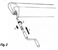
Unroll the awning while keeping the crank down. The awning will only open after a couple of turnings.
