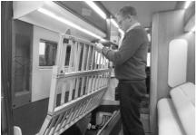
**Step 4:** Standing in the middle of the bed pull upward the sliding section of the frame..
