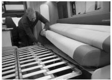
**Step 6:** Lowering the bed fame, ensure hooks locate into the off side bed base top
