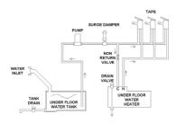
When power is supplied to the pump, it will draw water from the water tank, and pump it to the motorhome taps, shower and water heater.
