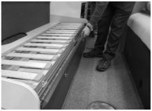
**Step 1:** Remove the Near side bed cushions and release the front facia flap at the top of the bed
