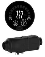
The Whale Heat Air is a dual fuel blown air space heater fitted beneath the motorhome. The controller mounted above the entrance door allows the selection of 230v / mains electric bottled gas energy sources to heat your motorhome, when they are available, along with selection of target room temperature. A 12v fan within the heater distributes heated air through the motorhome via furniture mounted outlets.
