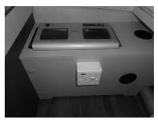
The water heater must not (and cannot) be used (heated) whilst en-route. Isolate the gas supply before starting your journey.
