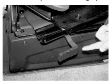
To turn the swivel, slide the BLACK lever rearwards and adjust to the required angle. Before driving off ensure the locking mechanism is fully secure.
