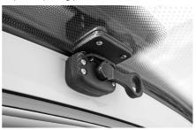
To close, turn the handle clockwise until the dome lies on the seal and a resistance is noticeable.
