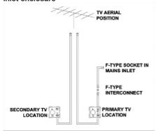
A short co-ax lead featuring a screw on co-ax connection will be present behind the Blue mains inlet connector. A co-ax cable will be fitted and connected within the motorhome, from the back of this connection, to the primary TV position within the motorhome. At the same time, further co-ax cable or cables will be fitted which route from the TV aerial position (i.e. within the wardrobe) to each of the TV positions within the motorhomes.
