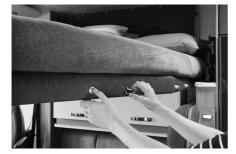
Please ensure the bed is fully returned to its 'up' position and that the release button has returned to its resting position before travelling.
