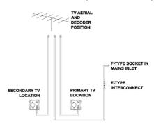
A short co-ax lead featuring a screw on co-ax connection will be present behind the Blue mains inlet connector. A co-ax cable will be fitted and connected within the motorhome, from the back of this connection, to the location intended for the later fitment of a satellite decoder or similar receiver. This external connection can be used to link an external dish or signal, to the decoder / receiver position.
