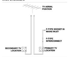
A short co-ax lead featuring a screw on co-ax connection will be present behind the Blue mains inlet connector. A co-ax cable will be fitted and connected within the motorhome, from the back of this connection, to the primary TV position within the motorhome. At the same time, further co-ax cable or cables will be fitted which route from a likely TV aerial position (i.e. within the wardrobe) to each of the TV positions within the motorhomes.
