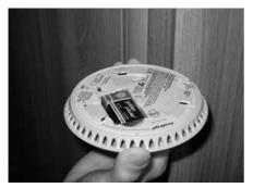
Replace the alarm on its mounting plate, lining up the large central vent on the front of the alarm, with the 'X' that is moulded into the plastic on the mounting plate (if unsure see page 13 of the alarm user manual). Ensure the unit is securely fitted.
