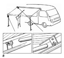
When raining, lower one side of the awning in such a way that the water can run down the fabric. Prevent the fabric from flying up by a sudden wind blow by using the hold down kit (optional).
