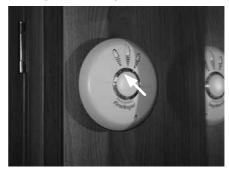
**Note:** The test button accurately tests the alarm's smoke sensing circuit, there is no need to test your alarm with smoke. If your smoke alarm fails to give an audible test signal, please refer immediately to the troubleshooting guide at the end of the user manual supplied.
