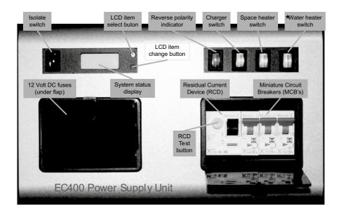
\* On conversions that use a combination space / water heater appliance the water heater button is not used.
