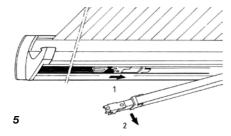
6. Adjust them to the required height. The fabric can be tightened by rolling up a little.
