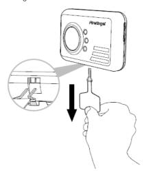
Your detector comes complete with an integrated power pack that will provide power for its entire operational life. To activate the power pack you need to pull the disabling tab (see image). This will in turn pull out the metal disabling clip, which is attached to the end of the tab, from the disabling socket which is situated on the underside of the detector. Retain the disabling tab for future use by taping it to page 20 of the CO-9X user manual.
