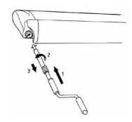
Unroll the awning while keeping the crank down. The awning will only open after a couple of turnings.
