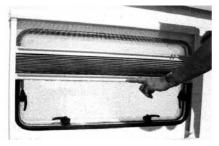
**Closing:** Grab the end bar in the middle and push the blind and flynet together or singly (blind - lower end bar) downwards until the required position is reached.
