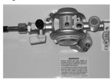
Your motorhome is supplied with a wall mounted gas regulator plumbed inside the gas cylinder compartment. The regulator and all appliances work at a harmonised 30mb pressure, which work with Butane and Propane gas.
