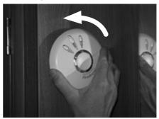
Remove the existing battery and replace with a new battery from the list on the previous page, making sure that the positive and negative connections are in the correct position. If unsure see the alarm user manual.
