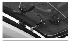
▲ WARNING: Before setting off, the vent must be shut and all catches engaged. To do this, pull the vent shut by the handles, press the buttons and turn them to engage the catches. Should the engine be started with the vent open, an audible warning will sound. Please be aware this warning will not alert the driver if the catches have not been properly engaged, only if the vent is left open when the engine is running.
