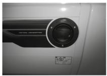
Use only unleaded petrol with the generator, the tank had a capacity of approx. 25 litres.
