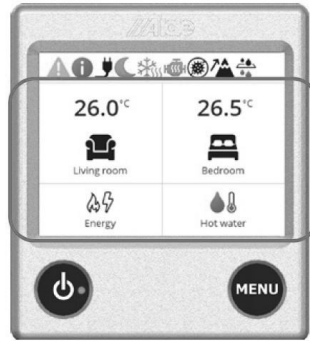
Control panel main menu screen
