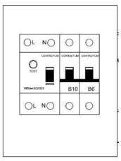
The consumer unit is located in the wardrobe, consists of one RCD and two MCB's, and operates in a similar way to components found in domestic installations.
