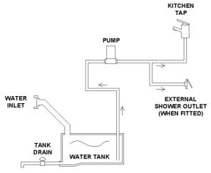
When power is supplied to the pump, it will draw water from the water tank, and pump it to the campervan kitchen tap and shower. The pump is fitted with its own pressure switch, and will continue to pump water, until the pressure of water on the output of the pump reaches a preset level. For this pressure to be achieved, the taps must be closed.
