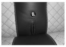
The top tether anchor points are located on the metal seat frame at the rear of the seat.
