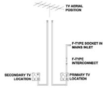
A short co-ax lead featuring a screw on co-ax connection will be present behind the Blue mains inlet connector. A co-ax cable will be fitted and connected within the motorhome, from the back of this connection, to the primary TV position within the motorhome. At the same time, further co-ax cable or cables will be fitted which route from a likely TV aerial position (i.e. within the wardrobe) to each of the TV positions within the motorhomes.
