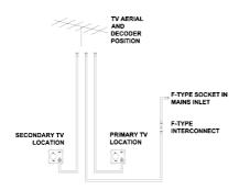
A short co-ax lead featuring a screw on co-ax connection will be present behind the Blue mains inlet connector. A co-ax cable will be fitted and connected within the motorhome, from the back of this connection, to the location intended for the later fitment of a satellite decoder or similar receiver. At the same time, further co-ax cable or cables will be fitted which route from a likely TV aerial position (i.e. within the wardrobe) to each of the TV positions within the motorhome.
