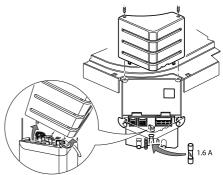
The water heater 12 V fuse is on the electronic control unit on the water heater.
