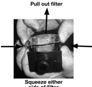
Squeeze either side of filter housing
