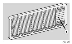
In winter, check that the ventilation grilles and the exhaust duct system (1) have not been blocked by snow, leaves, etc.
