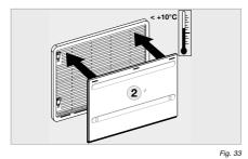
You should also attach the winter covers if the vehicle is taken out of service for a longer period of time or while it is being cleaned from the outside.
