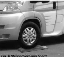
Fig. A Stepped levelling board
