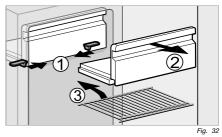
To enlarge the cooling compartment, just remove the freezer compartment.
