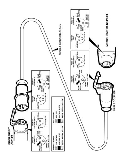
The legal length of the mains inlet cable is  $25 \pm 2$  metres. When in use it must be fully uncoiled and protected from traffic.
