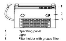
The extractor hood 524 serves to extract water vapour from cooking areas in motorhomes. The integrated halogen lamps (2) serve to illuminate the work surface.
