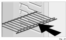
The storage racks may be pulled out by smoothly lifting them and may be positioned as desired.
