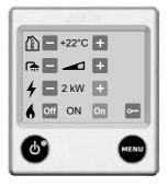
**Note:** if "Standby Brightness" is set to Off, the display goes out when it enters standby mode, but lights up if you press the screen. See settings under 9.12.
