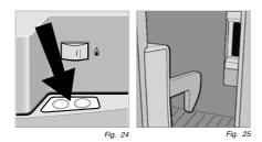
Open the door by pressing the locking button and pull open (see Fig. 24).
