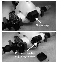
The pump may have to be removed to gain access to the adjusting screw. Drain the water system before removing the pump.
