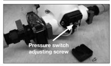
The pump may have to be removed to gain access to the adjusting screw. Drain the water system before removing the pump.
