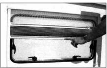
**Closing:** Grab the end bar in the middle and push the blind and flynet together or singly (blind - lower end bar) downwards until the required position is reached.
