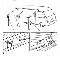
When raining, lower one side of the awning in such a way that the water can run down the fabric. Prevent the fabric from flying up by a sudden wind blow by using the hold down kit (optional).
