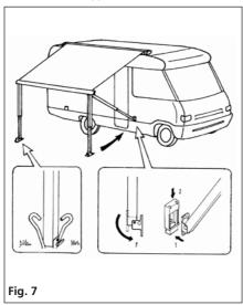
8. Install the tension rafter (for 3.75 m awning).
