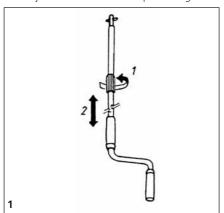
2. Introduce the crank arm into the bayonet joint.
