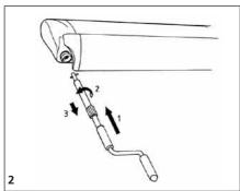
3. Unroll the awning while keeping the crank down. The awning will only open after a couple of turnings.
