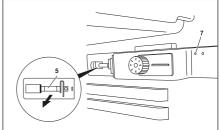
Slide in the new lamp between the sheet metal straps, until it snaps into place.
