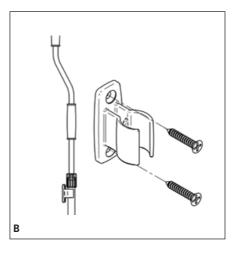
B. Install the bracket with the supplied screws or rivets
