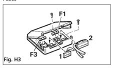
The device and control panel fuses are on the electronic control unit on the device.
