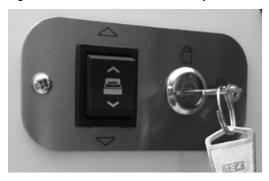
If fitted to your motorhome, the bed control panel will be positioned next to the main control panel located above the habitation entrance door.
