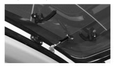
⚠ WARNING: Before setting off, the vent must be shut and all catches engaged. To do this, pull the vent shut by the handles, press the buttons and turn them to engage the catches. Should the engine be started with the vent open, an audible warning will sound. Please be aware this warning will not alert the driver if the catches have not been properly engaged, only if the vent is left open when the engine is running.
