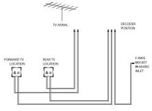
A short co-ax lead featuring a screw on co-ax connection will be present behind the Blue mains inlet connector. A co-ax cable will be fitted and connected within the motorhome, from the back of this connection, to the location intended for the later fitment of a satellite decoder or similar receiver. The external connection can be used to link an external dish or signal, to the decoder / receiver position.
