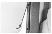
Catcher enables three positions of the window. Open position is where the handle is open placed on the outer part of the catcher. If the handle is placed in the middle of the catcher, this is position for ventilating. Closed position is position where the handle is closed on the inner part of the catcher.
