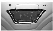
A large opening vent is provided in the luton bed area for ventilation purposes. To open the vent, press the buttons on the handles and turn the handles to release the catches. Once all the catches are released the vent will open until the gas struts restrict any further travel. Please note that the vent is only designed to open through a small angle.
