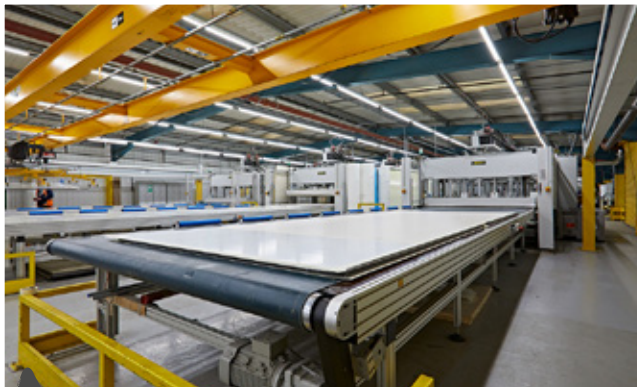
'SMART' GRP sidewall during the production process.
