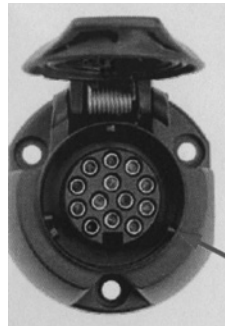
Fig. 5 - Socket body (containing female socket terminals) fitted to the car
