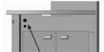
Typical 2nd thermostat and switch arrangement
