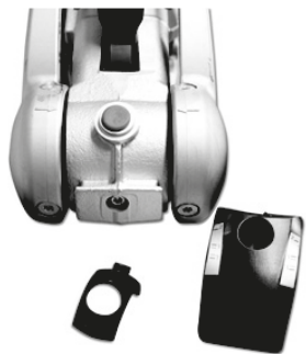
Fig 3. cheese head screw revealed
