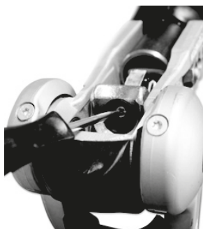
Fig 4. Remove head cap screw
