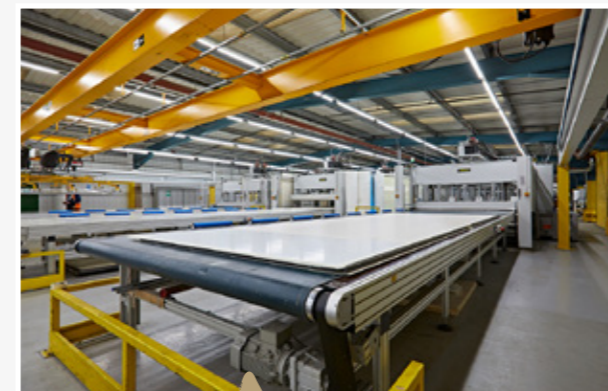
'SMART' GRP sidewall during the production process.
