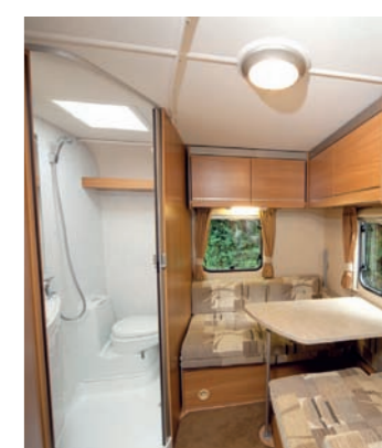
Washroom is compact with integral plastic tray floor and tambour door
