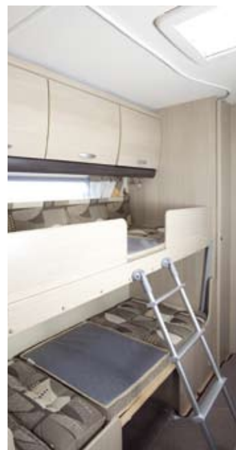
Side dinette converts into bunks at night. Aluminium ladder and plastic brackets feel substantial and guard wraps around to keep pillows in place
