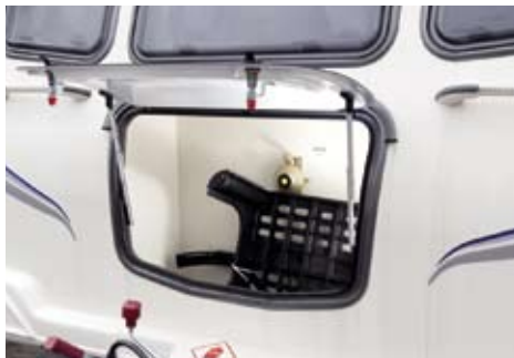
Front locker lid does not lift very high, making it difficult to manoeuvre gas bottles in and out
