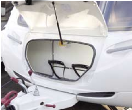
Gas support strut lifts lid high on spacious front locker for easy access to two gas bottles
