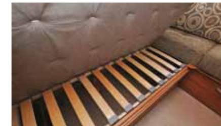
Beech slats are used for seat bases, but access underneath is via the tops only (no side access flaps).
