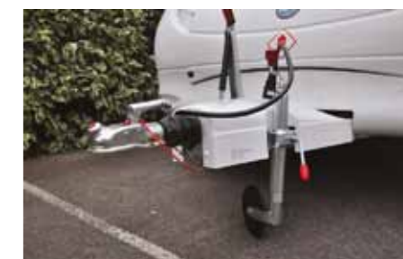
It's all simple - normal hitch, hand brake and jockey wheel - but it does the job.
