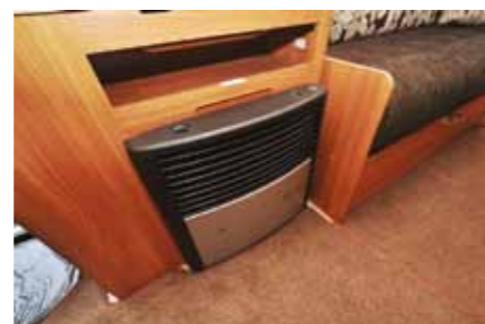
A Truma heater means you don't have to rely on the blown-air system for heating.
